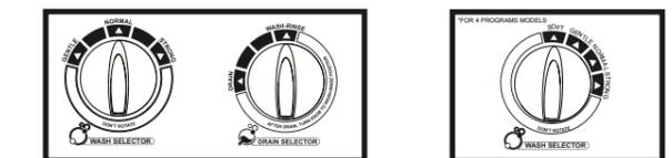
Set the desired wash time by turning the knob clockwise (refer table below for time selection)
